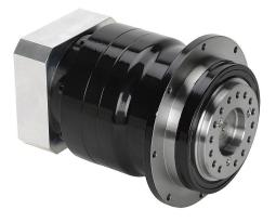
SureGear high-precision planetary gearbox, 50:1 ratio, inline with hub style output, nominal output torque 180 N-m (1593 lb-in), 2-stage, 110mm frame. For use with SureServo and SureServo2 SV(2)L-210(B) motors.
