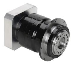
SureGear high-precision planetary gearbox, 35:1 ratio, inline with hub style output, nominal output torque 180 N-m (1593 lb-in), 2-stage, 110mm frame. For use with SureServo and SureServo2 SV(2)M-210(B) motors.
