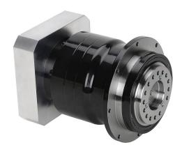
SureGear high-precision planetary gearbox, 25:1 ratio, inline with hub style output, nominal output torque 180 N-m (1593 lb-in), 2-stage, 110mm frame. For use with SureServo and SureServo2 SV(2)M-210(B) motors.
