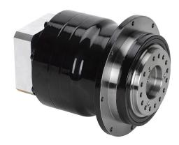
SureGear high-precision planetary gearbox, 25:1 ratio, inline with hub style output, nominal output torque 180 N-m (1593 lb-in), 2-stage, 110mm frame. For use with SureServo and SureServo2 SV(2)L-207(B) motors.
