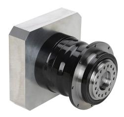
SureGear high-precision planetary gearbox, 10:1 ratio, inline with hub style output, nominal output torque 120 N-m (1062 lb-in), 1-stage, 110mm frame. For use with SureServo and SureServo2 SV(2)M-220(B) and SV(2)M-230(B) motors.
