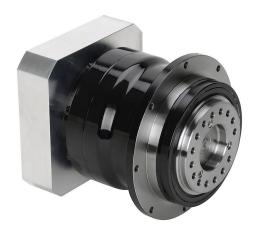
SureGear high-precision planetary gearbox, 10:1 ratio, inline with hub style output, nominal output torque 120 N-m (1062 lb-in), 1-stage, 110mm frame. For use with SureServo and SureServo2 SV(2)M-210(B) motors.
