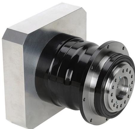
SureGear high-precision planetary gearbox, 5:1 ratio, inline with hub style output, nominal output torque 180 N-m (1593 lb-in), 1-stage, 110mm frame. For use with SureServo and SureServo2 SV(2)M-220(B) and SV(2)M-230(B) motors.
