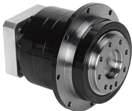
SureGear high-precision planetary gearbox, 25:1 ratio, inline with hub style output, nominal output torque 75 N-m (664 lb-in), 2-stage, 90mm frame. For use with SureServo and SureServo2 SV(2)L-202(B) and SV(2)L-204(B) motors.
