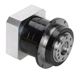
SureGear high-precision planetary gearbox, 10:1 ratio, inline with hub style output, nominal output torque 50 N-m (443 lb-in), 1-stage, 90mm frame. For use with SureServo and SureServo2 SV(2)L-210(B) motors.
