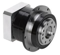
SureGear high-precision planetary gearbox, 10:1 ratio, inline with hub style output, nominal output torque 50 N-m (443 lb-in), 1-stage, 90mm frame. For use with SureServo and SureServo2 SV(2)L-207(B) motors.
