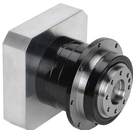
SureGear high-precision planetary gearbox, 5:1 ratio, inline with hub style output, nominal output torque 75 N-m (664 lb-in), 1-stage, 90mm frame. For use with SureServo and SureServo2 SV(2)M-210(B) motors.
