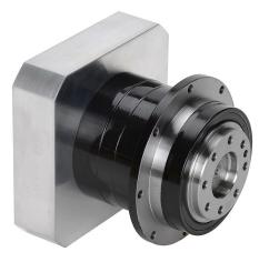
SureGear high-precision planetary gearbox, 5:1 ratio, inline with hub style output, nominal output torque 75 N-m (664 lb-in), 1-stage, 90mm frame. For use with SureServo and SureServo2 SV(2)M-210(B) motors.
