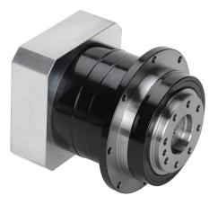
SureGear high-precision planetary gearbox, 5:1 ratio, inline with hub style output, nominal output torque 75 N-m (664 lb-in), 1-stage, 90mm frame. For use with SureServo and SureServo2 SV(2)L-210(B) motors.
