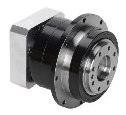
SureGear high-precision planetary gearbox, 5:1 ratio, inline with hub style output, nominal output torque 75 N-m (664 lb-in), 1-stage, 90mm frame. For use with SureServo and SureServo2 SV(2)L-207(B) motors.
