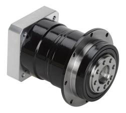
SureGear high-precision planetary gearbox, 25:1 ratio, inline with hub style output, nominal output torque 27 N-m (239 lb-in), 2-stage, 64mm frame. For use with SureServo and SureServo2 SV(2)L-202(B) and SV(2)L-204(B) motors.
