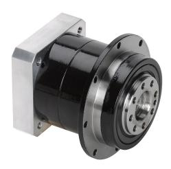
SureGear high-precision planetary gearbox, 10:1 ratio, inline with hub style output, nominal output torque 18 N-m (159 lb-in), 1-stage, 64mm frame. For use with SureServo and SureServo2 SV(2)L-202(B) and SV(2)L-204(B) motors.
