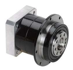
SureGear high-precision planetary gearbox, 10:1 ratio, inline with hub style output, nominal output torque 18 N-m (159 lb-in), 1-stage, 64mm frame. For use with SureServo and SureServo2 SV(2)L-202(B) and SV(2)L-204(B) motors.
