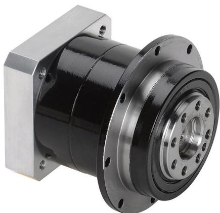
SureGear high-precision planetary gearbox, 5:1 ratio, inline with hub style output, nominal output torque 27 N-m (239 lb-in), 1-stage, 64mm frame. For use with SureServo and SureServo2 SV(2)L-202(B) and SV(2)L-204(B) motors.
