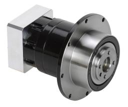
SureGear high-precision planetary gearbox, 25:1 ratio, inline with hub style output, nominal output torque 9 N-m (80 lb-in), 2-stage, 47mm frame. For use with SureServo and SureServo2 SV(2)L-201(B) motors.
