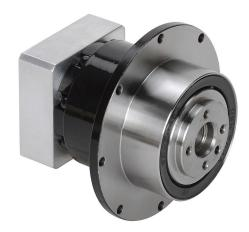
SureGear high-precision planetary gearbox, 10:1 ratio, inline with hub style output, nominal output torque 6 N-m (53 lb-in), 1-stage, 47mm frame. For use with SureServo and SureServo2 SV(2)L-201(B) motors.
