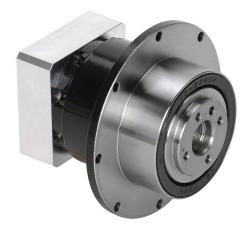
SureGear high-precision planetary gearbox, 5:1 ratio, inline with hub style output, nominal output torque 9 N-m (80 lb-in), 1-stage, 47mm frame. For use with SureServo and SureServo2 SV(2)L-201(B) motors.
