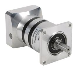
SureGear precision planetary gearbox, 100:1 ratio, inline, 0.375in diameter output shaft, nominal output torque 5 N-m (44 lb-in), 2-stage, NEMA 23 frame. For use with SureStep NEMA 23 motors.
