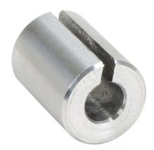
SureGear motor shaft bushing, for use with SureGear NEMA 17 gearboxes with 5mm diameter motor shaft.
