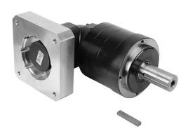
SureGear high-precision planetary gearbox, 25:1 ratio, right angle, 40mm diameter output shaft, nominal output torque 300 N-m (2655 lb-in), 3-stage, 155mm frame. For use with SureServo and SureServo2 SV(2)M-220(B) motors.
