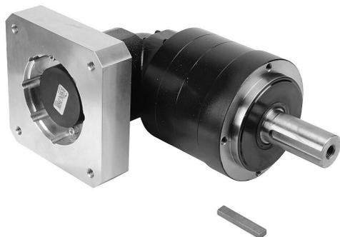
SureGear high-precision planetary gearbox, 25:1 ratio, right angle, 40mm diameter output shaft, nominal output torque 300 N-m (2655 lb-in), 3-stage, 155mm frame. For use with SureServo and SureServo2 SV(2)M-220(B) motors.
