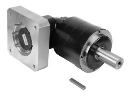
SureGear high-precision planetary gearbox, 15:1 ratio, right angle, 40mm diameter output shaft, nominal output torque 200 N-m (1770 lb-in), 3-stage, 155mm frame. For use with SureServo and SureServo2 SV(2)M-220(B) motors.
