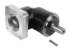
SureGear high-precision planetary gearbox, 5:1 ratio, right angle, 40mm diameter output shaft, nominal output torque 200 N-m (1770 lb-in), 2-stage, 155mm frame. For use with SureServo and SureServo2 SV(2)M-220(B) and SV(2)M-230(B) motors.
