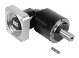
SureGear high-precision planetary gearbox, 25:1 ratio, right angle, 32mm diameter output shaft, nominal output torque 150 N-m (1328 lb-in), 3-stage, 120mm frame. For use with SureServo and SureServo2 SV(2)M-210(B) motors.
