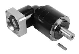
SureGear high-precision planetary gearbox, 25:1 ratio, right angle, 32mm diameter output shaft, nominal output torque 150 N-m (1328 lb-in), 3-stage, 120mm frame. For use with SureServo and SureServo2 SV(2)L-210(B) motors.
