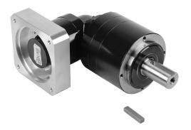
SureGear high-precision planetary gearbox, 15:1 ratio, right angle, 32mm diameter output shaft, nominal output torque 110 N-m (974 lb-in), 3-stage, 120mm frame. For use with SureServo and SureServo2 SV(2)M-210(B) motors.
