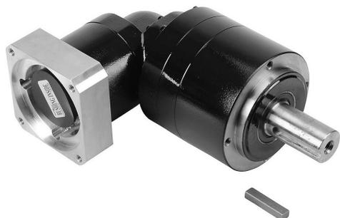
SureGear high-precision planetary gearbox, 15:1 ratio, right angle, 32mm diameter output shaft, nominal output torque 110 N-m (974 lb-in), 3-stage, 120mm frame. For use with SureServo and SureServo2 SV(2)L-210(B) motors.
