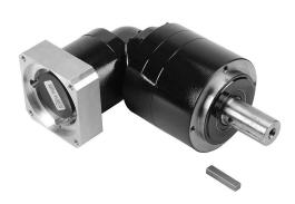
SureGear high-precision planetary gearbox, 15:1 ratio, right angle, 32mm diameter output shaft, nominal output torque 110 N-m (974 lb-in), 3-stage, 120mm frame. For use with SureServo and SureServo2 SV(2)L-210(B) motors.
