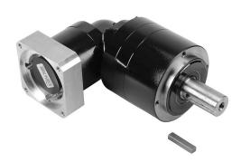
SureGear high-precision planetary gearbox, 15:1 ratio, right angle, 32mm diameter output shaft, nominal output torque 110 N-m (974 lb-in), 3-stage, 120mm frame. For use with SureServo and SureServo2 SV(2)L-210(B) motors.
