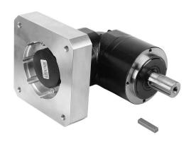
SureGear high-precision planetary gearbox, 10:1 ratio, right angle, 32mm diameter output shaft, nominal output torque 110 N-m (974 lb-in), 2-stage, 120mm frame. For use with SureServo and SureServo2 SV(2)M-220(B) and SV(2)M-230(B) motors.
