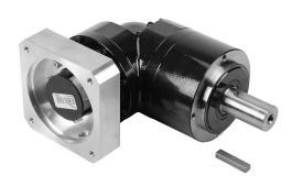
SureGear high-precision planetary gearbox, 10:1 ratio, right angle, 32mm diameter output shaft, nominal output torque 110 N-m (974 lb-in), 2-stage, 120mm frame. For use with SureServo and SureServo2 SV(2)M-210(B) motors.
