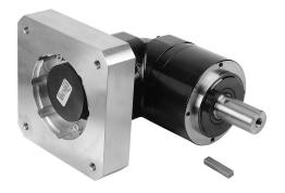
SureGear high-precision planetary gearbox, 5:1 ratio, right angle, 32mm diameter output shaft, nominal output torque 120 N-m (1062 lb-in), 2-stage, 120mm frame. For use with SureServo and SureServo2 SV(2)M-220(B) and SV(2)M-230(B) motors.
