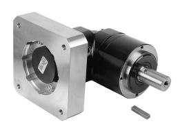
SureGear high-precision planetary gearbox, 5:1 ratio, right angle, 32mm diameter output shaft, nominal output torque 120 N-m (1062 lb-in), 2-stage, 120mm frame. For use with SureServo and SureServo2 SV(2)M-220(B) and SV(2)M-230(B) motors.
