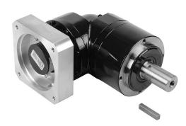
SureGear high-precision planetary gearbox, 5:1 ratio, right angle, 32mm diameter output shaft, nominal output torque 120 N-m (1062 lb-in), 2-stage, 120mm frame. For use with SureServo and SureServo2 SV(2)M-210(B) motors.
