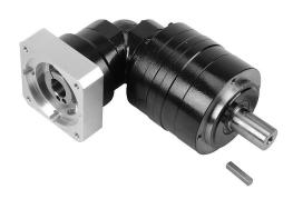
SureGear high-precision planetary gearbox, 25:1 ratio, right angle, 22mm diameter output shaft, nominal output torque 65 N-m (575 lb-in), 3-stage, 90mm frame. For use with SureServo and SureServo2 SV(2)L-207(B) motors.
