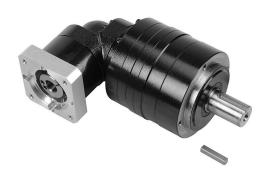
SureGear high-precision planetary gearbox, 25:1 ratio, right angle, 22mm diameter output shaft, nominal output torque 65 N-m (575 lb-in), 3-stage, 90mm frame. For use with SureServo and SureServo2 SV(2)L-202(B) and SV(2)L-204(B) motors.
