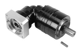
SureGear high-precision planetary gearbox, 15:1 ratio, right angle, 22mm diameter output shaft, nominal output torque 45 N-m (398 lb-in), 3-stage, 90mm frame. For use with SureServo and SureServo2 SV(2)L-207(B) motors.
