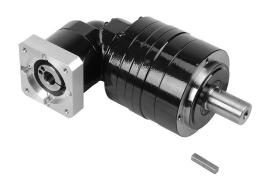
SureGear high-precision planetary gearbox, 15:1 ratio, right angle, 22mm diameter output shaft, nominal output torque 45 N-m (398 lb-in), 3-stage, 90mm frame. For use with SureServo and SureServo2 SV(2)L-202(B) and SV(2)L-204(B) motors.
