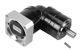
SureGear high-precision planetary gearbox, 10:1 ratio, right angle, 22mm diameter output shaft, nominal output torque 45 N-m (398 lb-in), 2-stage, 90mm frame. For use with SureServo and SureServo2 SV(2)L-210(B) motors.
