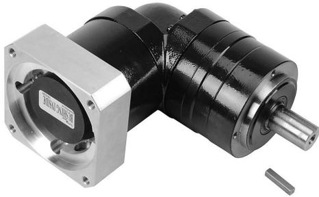
SureGear high-precision planetary gearbox, 10:1 ratio, right angle, 22mm diameter output shaft, nominal output torque 45 N-m (398 lb-in), 2-stage, 90mm frame. For use with SureServo and SureServo2 SV(2)L-210(B) motors.
