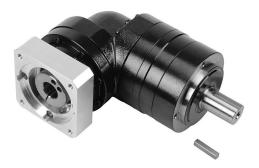
SureGear high-precision planetary gearbox, 10:1 ratio, right angle, 22mm diameter output shaft, nominal output torque 45 N-m (398 lb-in), 2-stage, 90mm frame. For use with SureServo and SureServo2 SV(2)L-207(B) motors.
