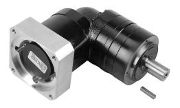
SureGear high-precision planetary gearbox, 5:1 ratio, right angle, 22mm diameter output shaft, nominal output torque 65 N-m (575 lb-in), 2-stage, 90mm frame. For use with SureServo and SureServo2 SV(2)L-210(B) motors.
