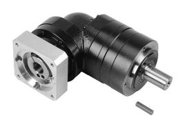
SureGear high-precision planetary gearbox, 5:1 ratio, right angle, 22mm diameter output shaft, nominal output torque 65 N-m (575 lb-in), 2-stage, 90mm frame. For use with SureServo and SureServo2 SV(2)L-207(B) motors.
