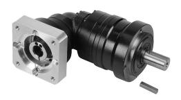
SureGear high-precision planetary gearbox, 25:1 ratio, right angle, 16mm diameter output shaft, nominal output torque 24 N-m (212 lb-in), 3-stage, 70mm frame. For use with SureServo and SureServo2 SV(2)L-202(B) and SV(2)L-204(B) motors.
