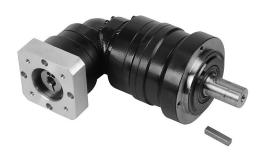
SureGear high-precision planetary gearbox, 25:1 ratio, right angle, 16mm diameter output shaft, nominal output torque 24 N-m (212 lb-in), 3-stage, 70mm frame. For use with SureServo and SureServo2 SV(2)L-201(B) motors.
