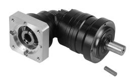
SureGear high-precision planetary gearbox, 15:1 ratio, right angle, 16mm diameter output shaft, nominal output torque 16 N-m (142 lb-in), 3-stage, 70mm frame. For use with SureServo and SureServo2 SV(2)L-202(B) and SV(2)L-204(B) motors.
