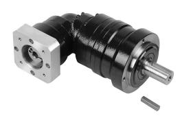
SureGear high-precision planetary gearbox, 15:1 ratio, right angle, 16mm diameter output shaft, nominal output torque 16 N-m (142 lb-in), 3-stage, 70mm frame. For use with SureServo and SureServo2 SV(2)L-201(B) motors.
