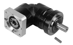
SureGear high-precision planetary gearbox, 10:1 ratio, right angle, 16mm diameter output shaft, nominal output torque 16 N-m (142 lb-in), 2-stage, 70mm frame. For use with SureServo and SureServo2 SV(2)L-202(B) and SV(2)L-204(B) motors.
