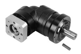
SureGear high-precision planetary gearbox, 10:1 ratio, right angle, 16mm diameter output shaft, nominal output torque 16 N-m (142 lb-in), 2-stage, 70mm frame. For use with SureServo and SureServo2 SV(2)L-201(B) motors.
