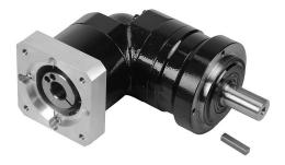
SureGear high-precision planetary gearbox, 5:1 ratio, right angle, 16mm diameter output shaft, nominal output torque 22 N-m (195 lb-in), 2-stage, 70mm frame. For use with SureServo and SureServo2 SV(2)L-202(B) and SV(2)L-204(B) motors.
