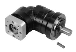
SureGear high-precision planetary gearbox, 5:1 ratio, right angle, 16mm diameter output shaft, nominal output torque 22 N-m (195 lb-in), 2-stage, 70mm frame. For use with SureServo and SureServo2 SV(2)L-201(B) motors.
