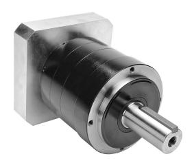
SureGear high-precision planetary gearbox, 15:1 ratio, inline, 40mm diameter output shaft, nominal output torque 240 N-m (2124 lb-in), 2-stage, 155mm frame. For use with SureServo and SureServo2 SV(2)M-220(B) and SV(2)M-230(B) motors.
