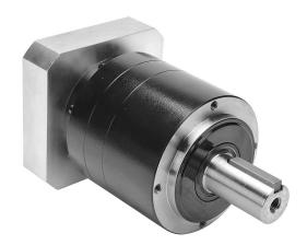
SureGear high-precision planetary gearbox, 25:1 ratio, inline, 32mm diameter output shaft, nominal output torque 180 N-m (1593 lb-in), 2-stage, 120mm frame. For use with SureServo and SureServo2 SV(2)M-210(B) motors.
